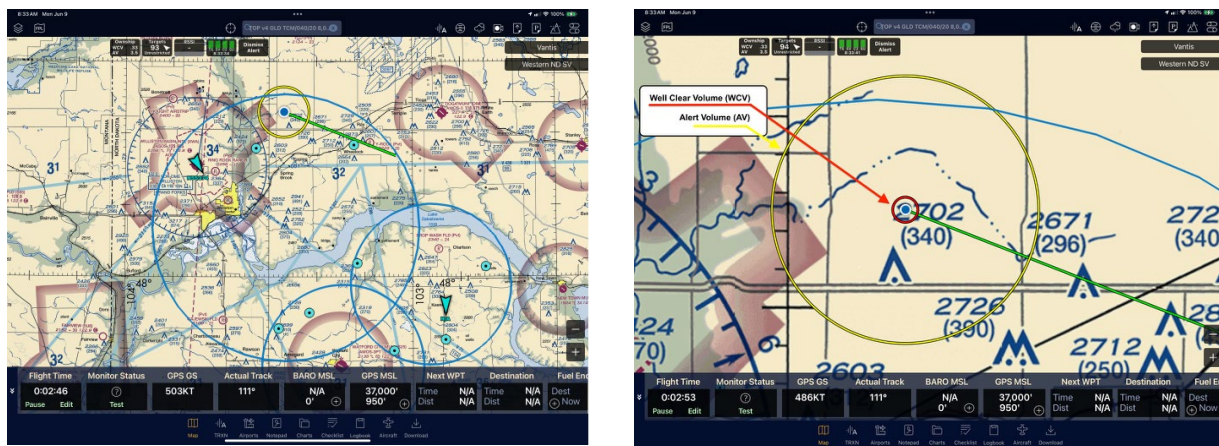
Figure 6: Examples of UAS Ownship Displayed on a Flight Crew HMI (left) and the DAA Alert Volume (yellow, outer ring) and the DAA Well Clear Volume (red, inner ring) (right)
