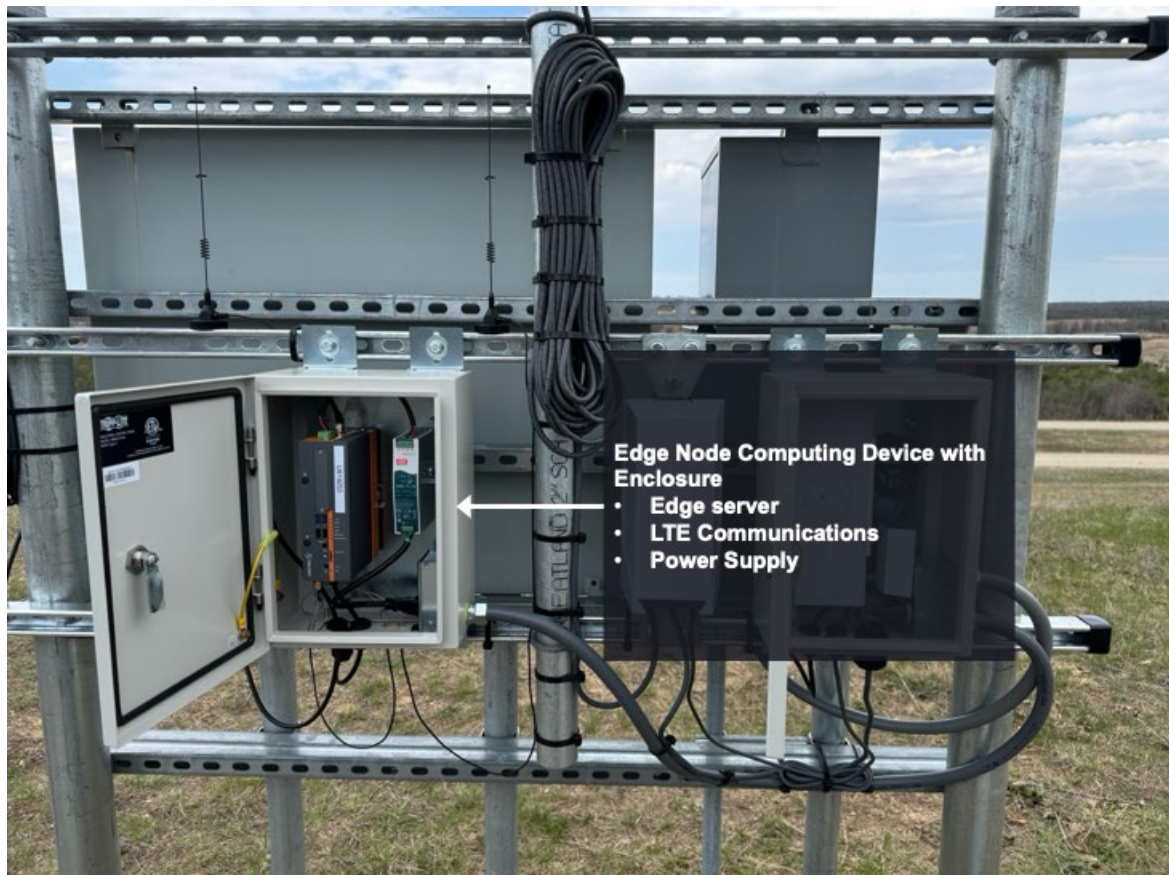
Figure 11: (Example) Edge Node Comprising an Edge Server, Built-in LTE, and Power Supply
